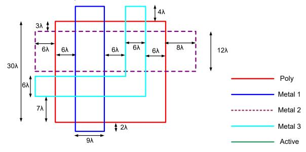
Problem 4 Design a 3K resistor in the 0.5μm CMOS process. Use Poly 1 with a silicide block for the resistor (designated as HR-POLY). The width-length ratio of an
